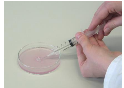
Figure 1: Injection of gas mixture into a soap solution
