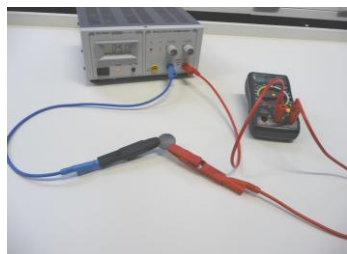
Fig.1 Set-up of E1. For E2 a piece of tungsten wire is used instead of the silicon plate.
