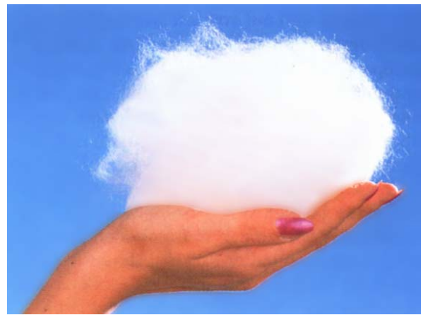
Fiberfill for anoraks; silicone emulsions help them resist laundering and dry cleaning
